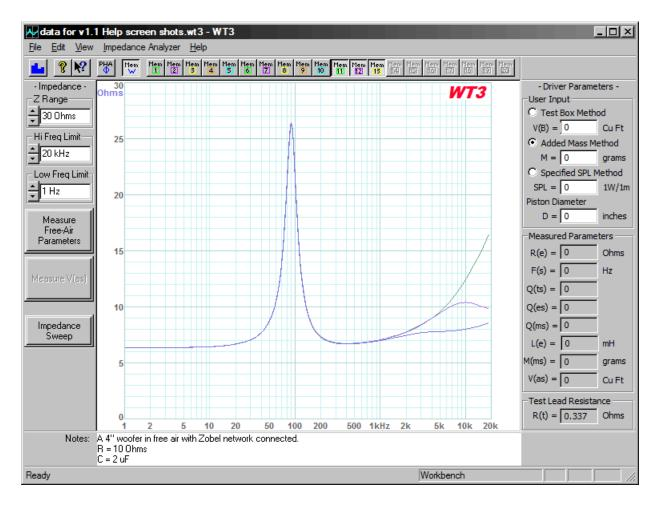
The screen below shows the effect of increasing the capacitor to 3 uF (blue trace). The increase from 2 to 3 uF gave even further improvement as the impedance above resonance is now quite flat. Just to see what happens, let's increase the capacitor further to 5 uF.
